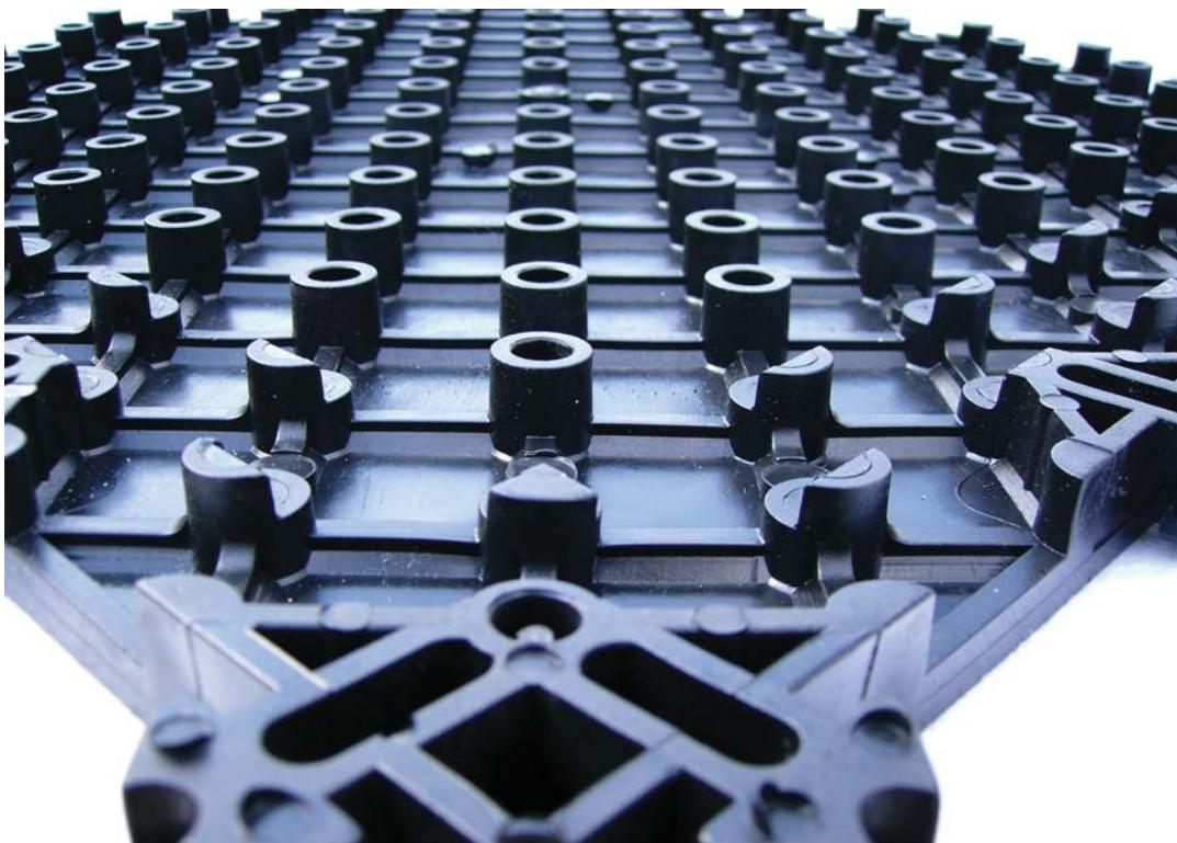
The innovative feature of Matta Safety Surfacing is the network of evenly spaced compression columns located on the underside of all Matta tiles. These pliable columns act as springs when weight is applied to the surface of the tile, the columns compress to provide a comfortable degree of cushion, while maintaining proper support and alignment for the skeletal structure.
