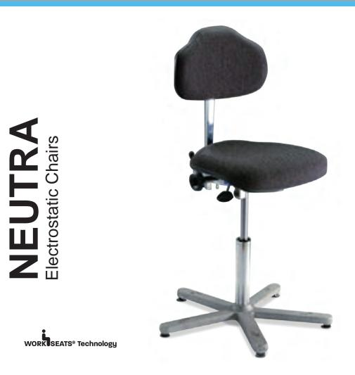
Fabric or vinyl conductive seating mounted on a five star cast aluminum base equipped with conductive glides or conductive self-braking casters that provide maximum dissipation of electro-static discharges. As with all Milagon seating systems the Neutraseries chair conforms with the ergonomic and safety requirements prescribed by ANSI/BIFMA.
